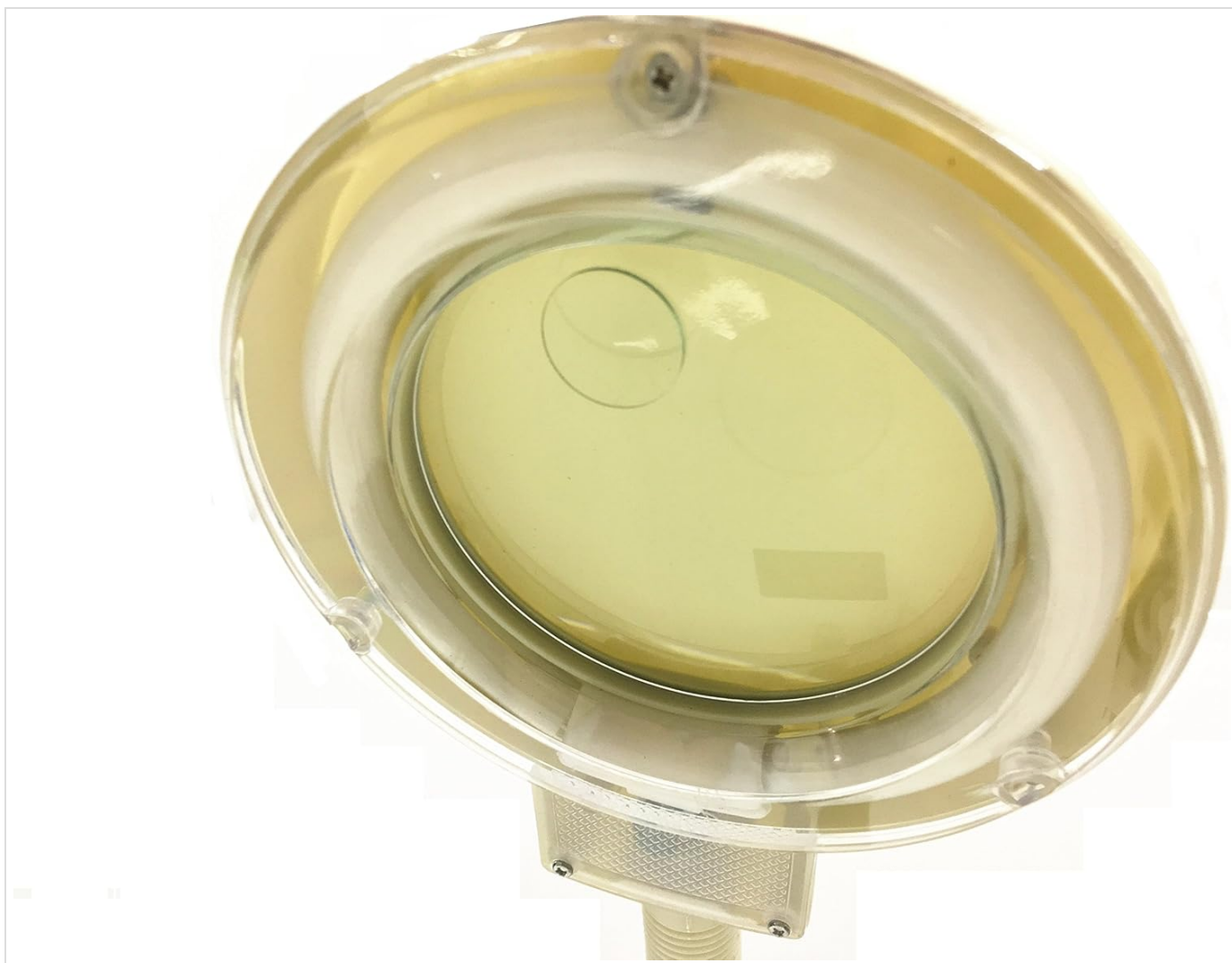
Figure 3: Magnifying lens and counting plate. This shows the illuminated area where petri dishes are placed for colony counting, with the magnifying lens positioned above.
