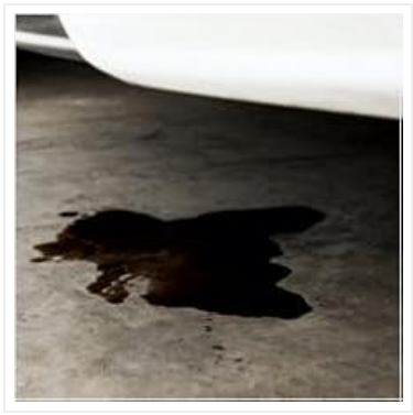
Image 6.1: An oil stain on a garage floor, indicating a potential engine oil leak that a new valve cover gasket aims to prevent.
