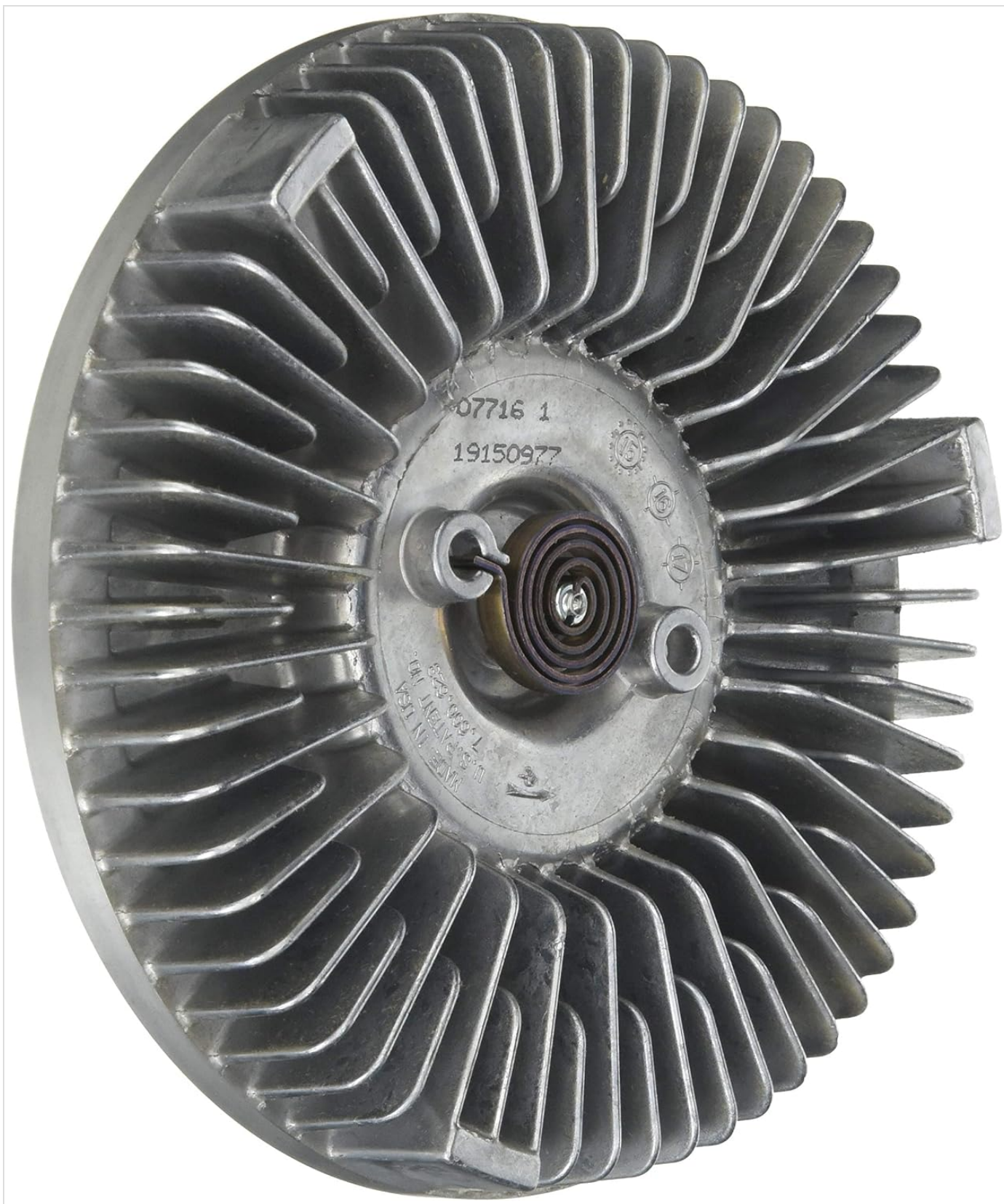
Figure 2: Rear view of the GM Genuine 19150977 Fan Blade Clutch. This image highlights the rear side of the clutch, featuring the bimetallic thermal spring mechanism at its center, which controls the clutch engagement. Several bolt holes for attaching the fan blades are also visible around the perimeter.
