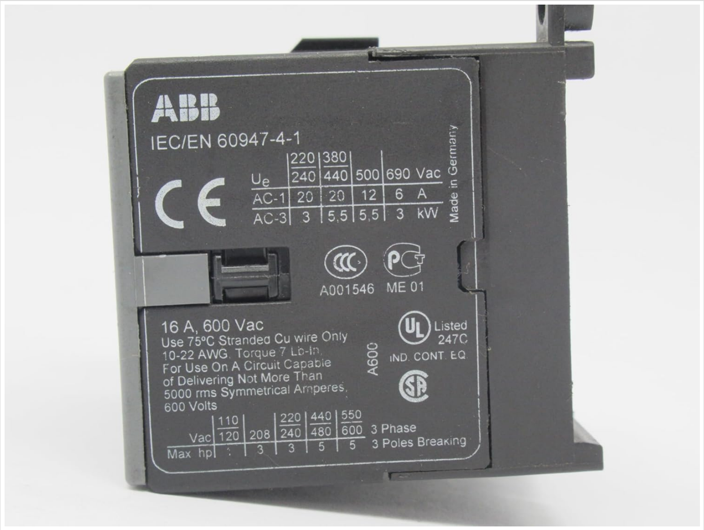
Figure 4: Bottom view of the ABB B7-30-10-01 Mini Contactor, displaying the technical specifications label. This label provides critical information such as IEC/EN 60947-4-1 compliance, rated operational voltage (Ue), AC-1 and AC-3 current ratings, power ratings (kW), UL listing, and maximum horsepower ratings for various voltages and phases.
