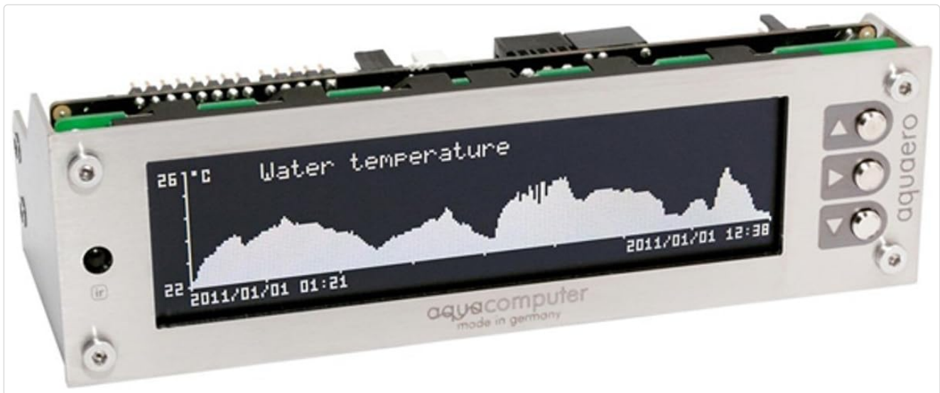
Image 1.1: Front view of the Aquacomputer Aquaero 6 PRO, showing the graphic LCD and control buttons. The display indicates water temperature readings over time.
