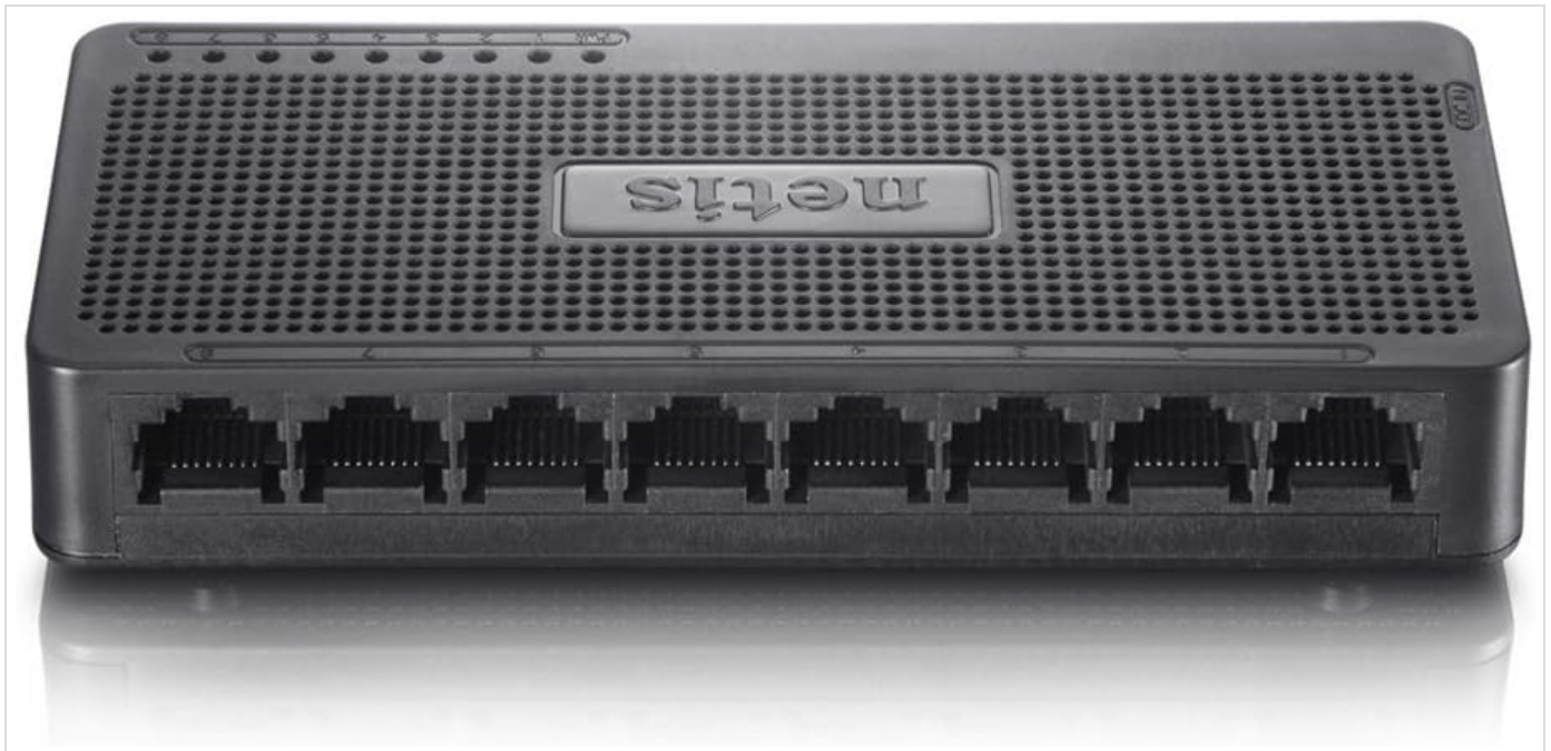
Figure 3.1: Front view of the Netis ST3108S switch.
