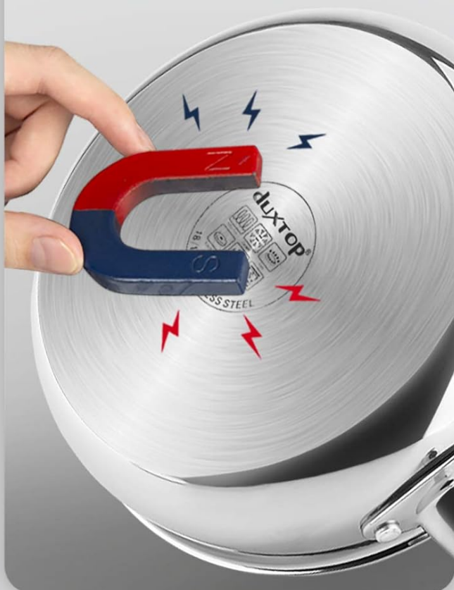
Figure 2: Cookware Compatibility Test
