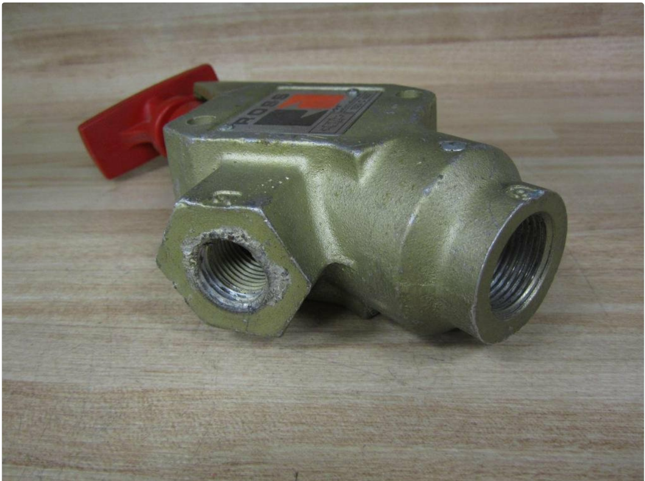
Figure 4.1: Side view of the Ross 1523C4002 valve, highlighting the threaded ports for connection to pneumatic systems.
