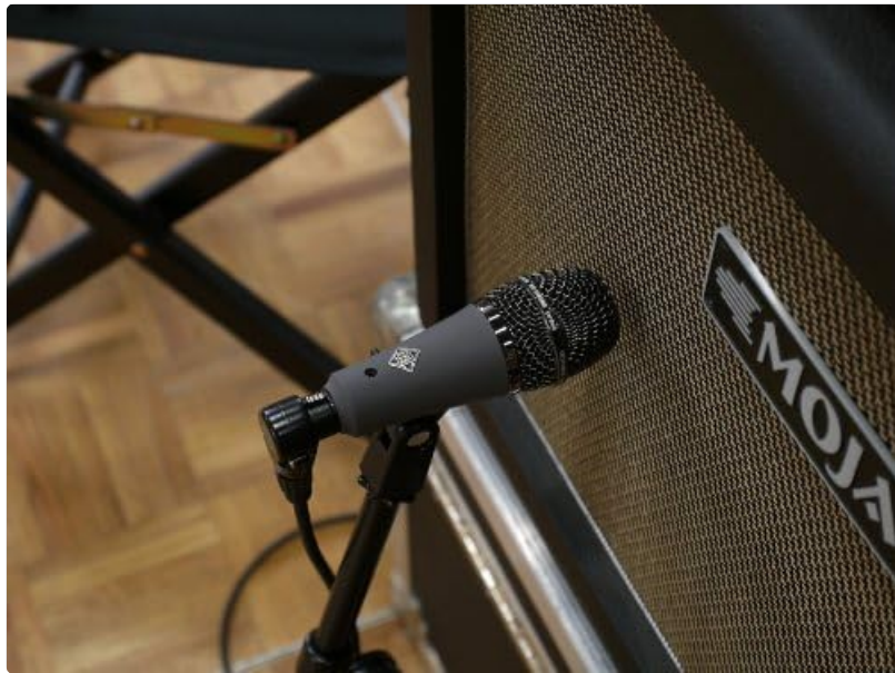
Image: The TELEFUNKEN M81-SH microphone positioned on a stand, ready to capture sound from a guitar amplifier. This illustrates a typical setup for instrument recording.
