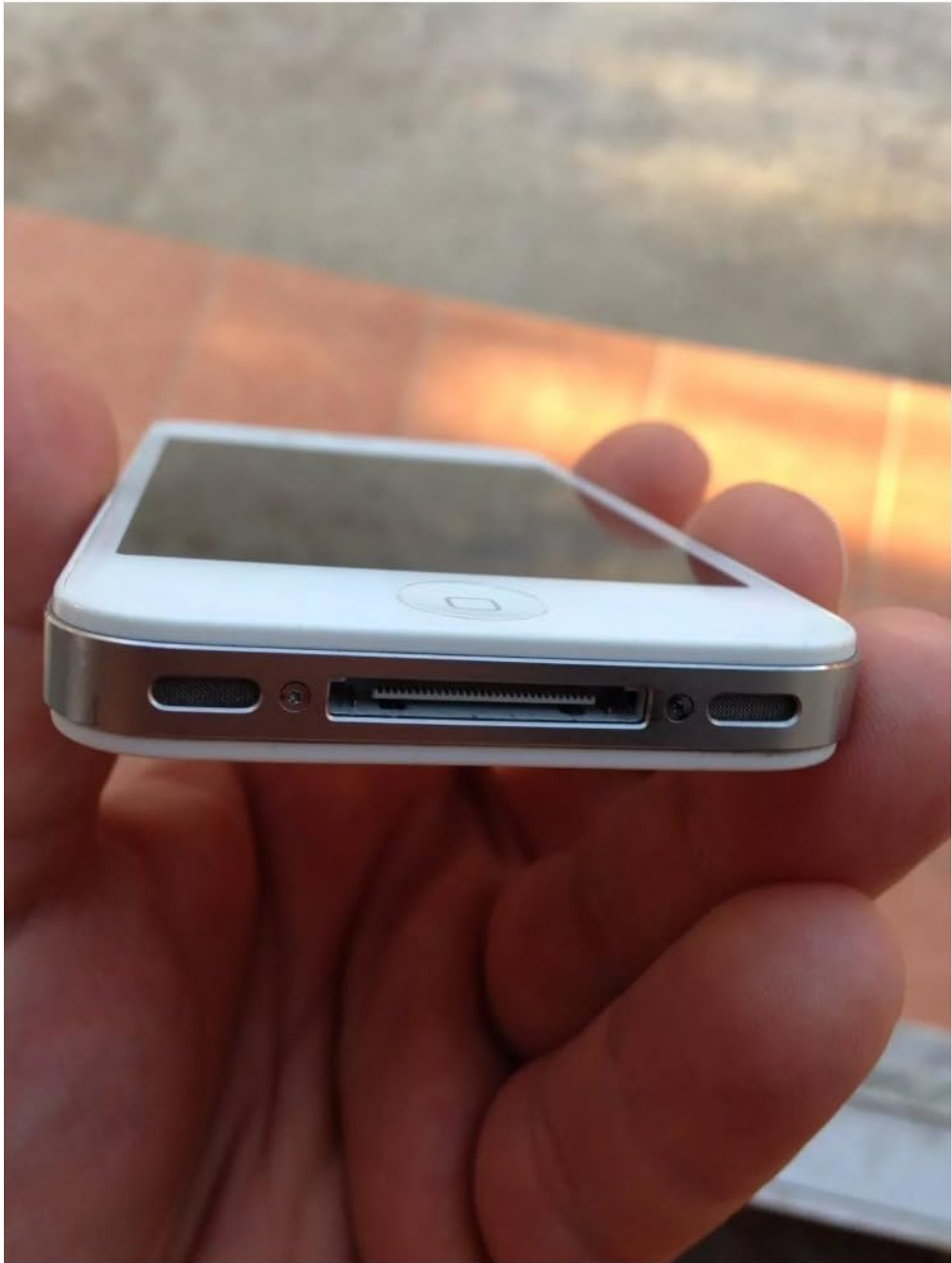
Image: Bottom view of the iPhone 4S, showing the 30-pin dock connector and speaker grilles.
