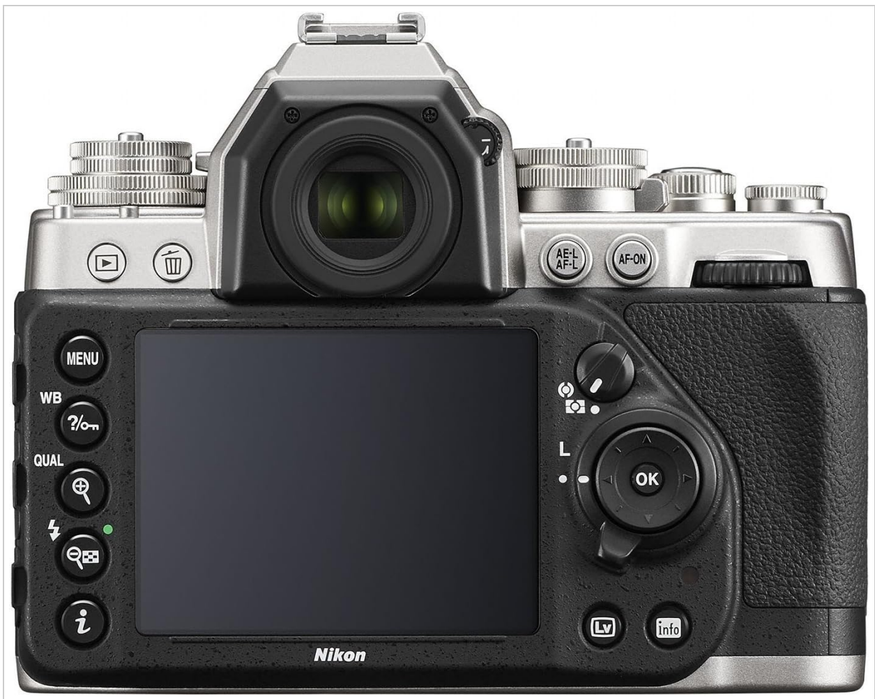
Rear view of the Nikon Df, showing the LCD screen, navigation buttons, and the optical viewfinder.
