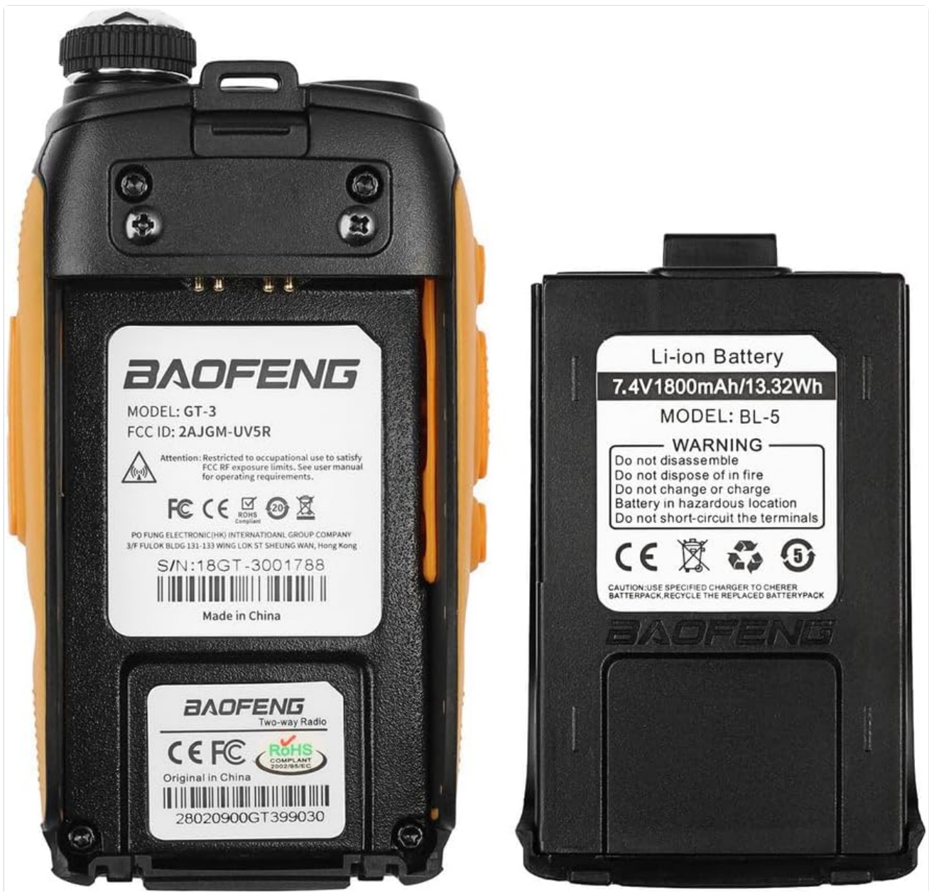
Image 4: The 7.4V 1800mAh Li-ion Battery Pack.
