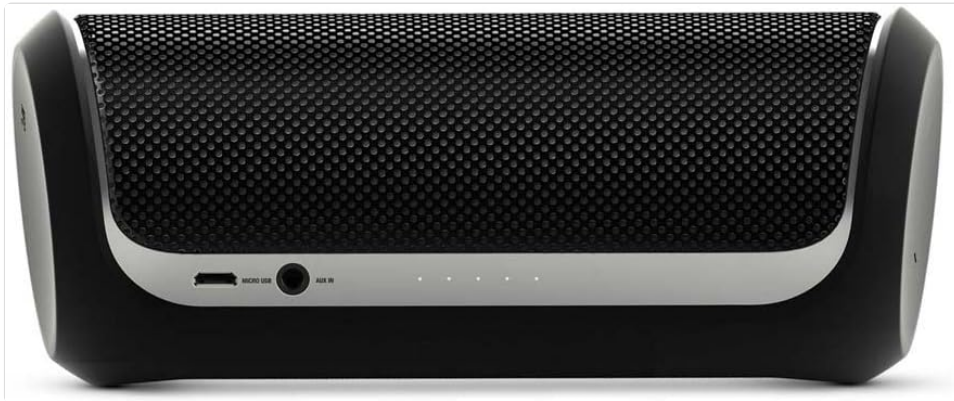
Figure 4.1: Rear view of the JBL Flip 2 showing charging and auxiliary ports.
