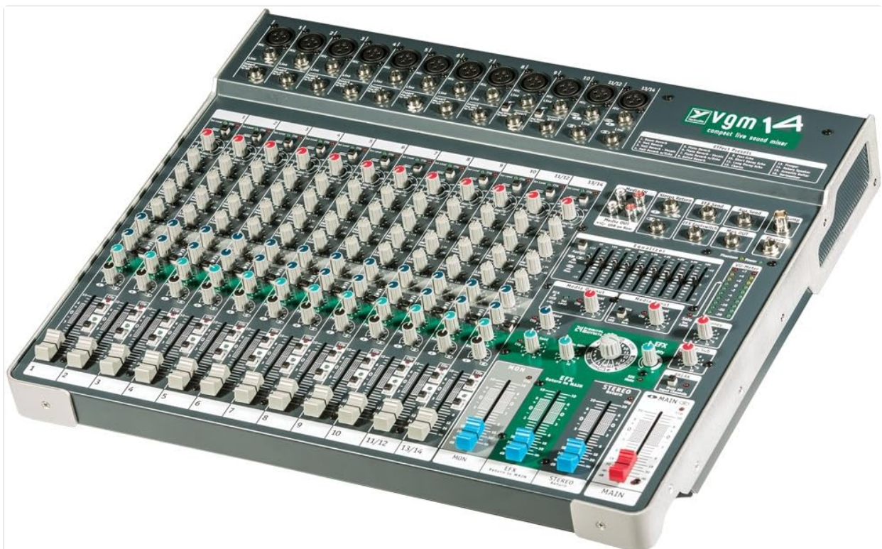
Figure 3: Angled View of Mixer. This image provides an angled perspective of the Yorkville VGM14 mixer, showcasing the overall design and the accessibility of its various controls, including the channel strips, master section, and graphic equalizer.
