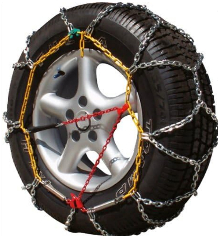
Figure 1: Green Valley Xtragrip N°110 snow chain correctly installed on a vehicle tire. This image demonstrates the pattern of the chains across the tread and the attachment points around the wheel.
