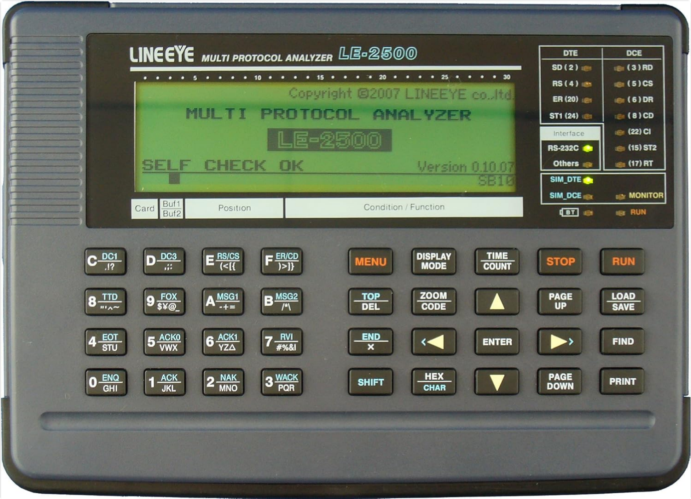
Figure 3.1: Front view of the LE-2500-E Multi Protocol Analyzer, showing the display screen, keypad, and interface indicators.
