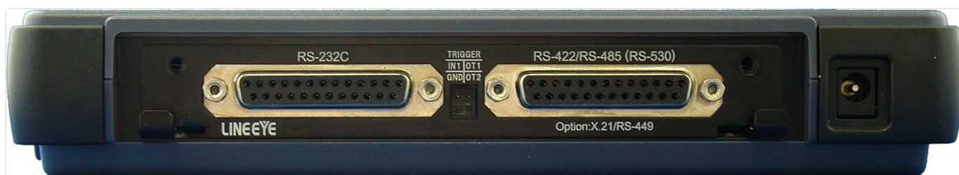
Figure 4.2: Rear view of the LE-2500-E, showing the RS-232C and RS-422/485 (RS-530) communication ports. Note the TRIGGER input for external synchronization.
