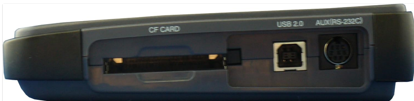
Figure 4.3: Side view of the LE-2500-E, illustrating the CF card slot, USB 2.0 port, and AUX (RS-232C) port.
