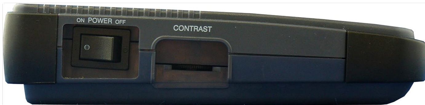
Figure 4.1: Side view of the LE-2500-E, highlighting the ON/OFF power switch and the contrast adjustment knob.
