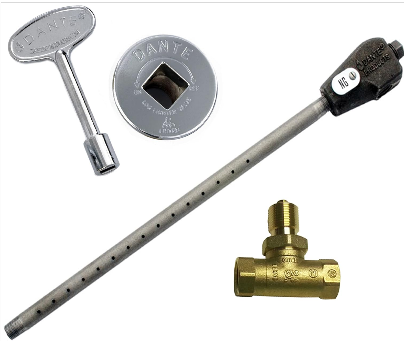
Figure 1: Overview of the Dante Universal Log Lighter Combo Kit components. This image displays all parts included in the kit: a chrome-plated key for operating the valve, a circular chrome floor plate that covers the valve opening, a long metal tube which is the natural gas log lighter with an attached mixer at one end, and a brass T-fitting for gas line connection.
