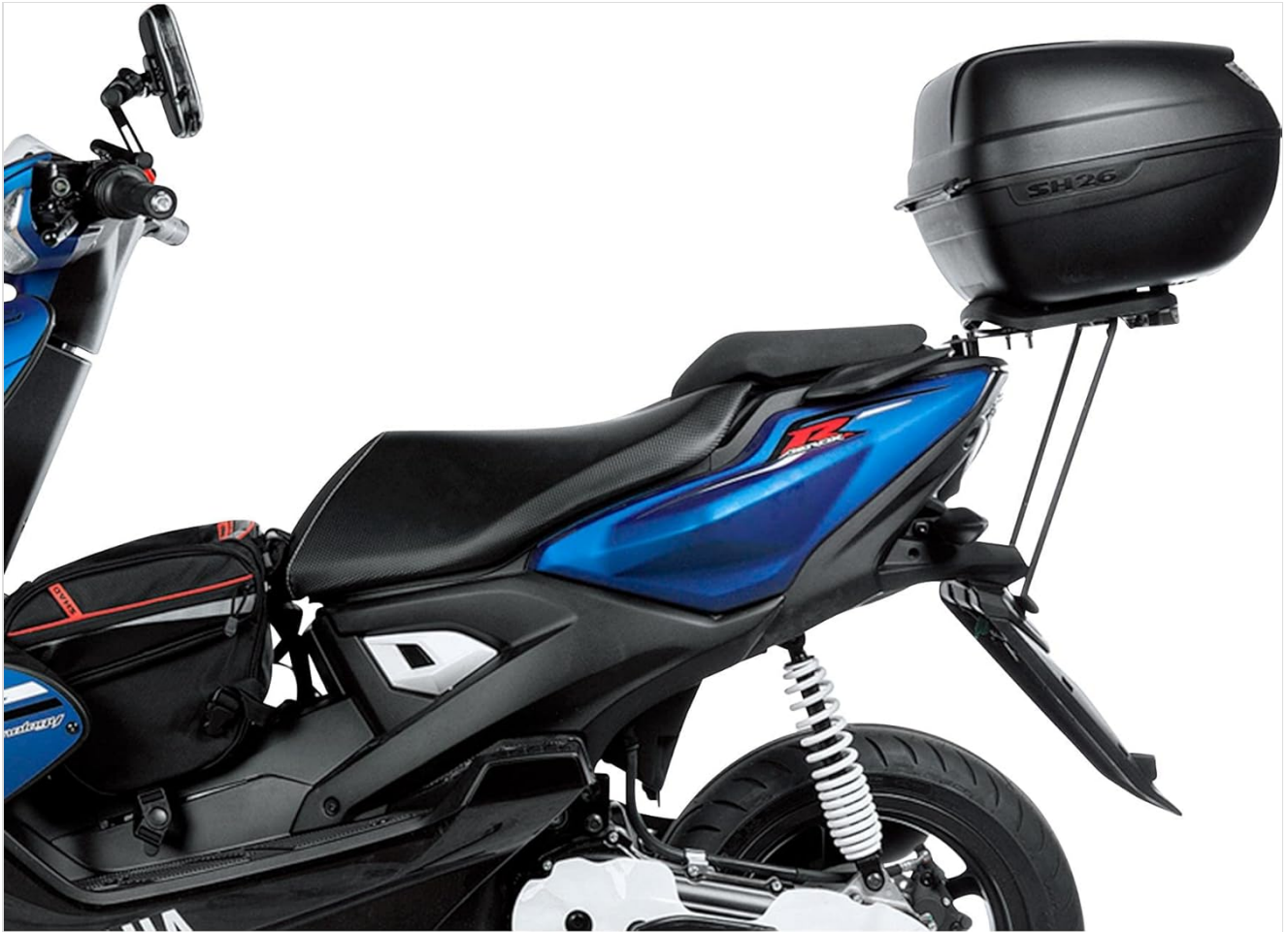
Figure 3.3: The fitting kit with a SHAD SH26 top case mounted, illustrating compatibility with various SHAD top case models.
