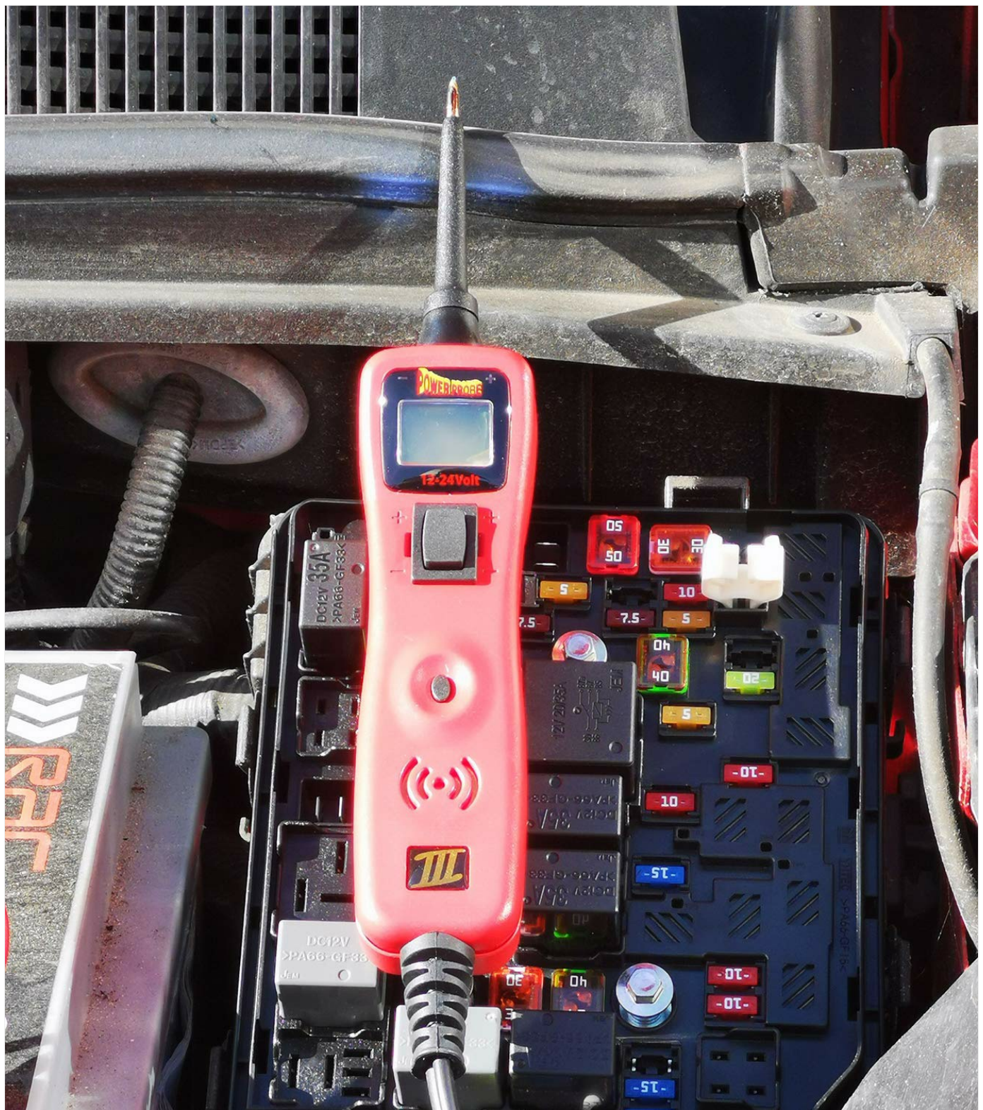
Figure 5: The Power Probe III being used to test circuits within a vehicle's fuse box, demonstrating its application in diagnosing electrical faults.
