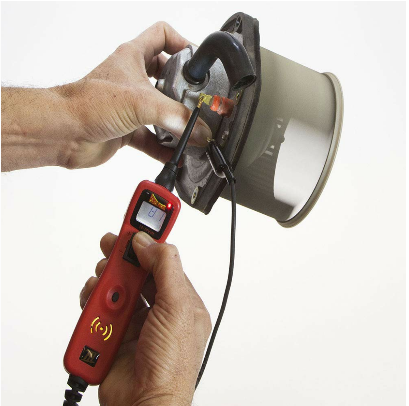
Figure 4: A technician using the Power Probe III to test an automotive component, demonstrating its ability to apply power or ground.
