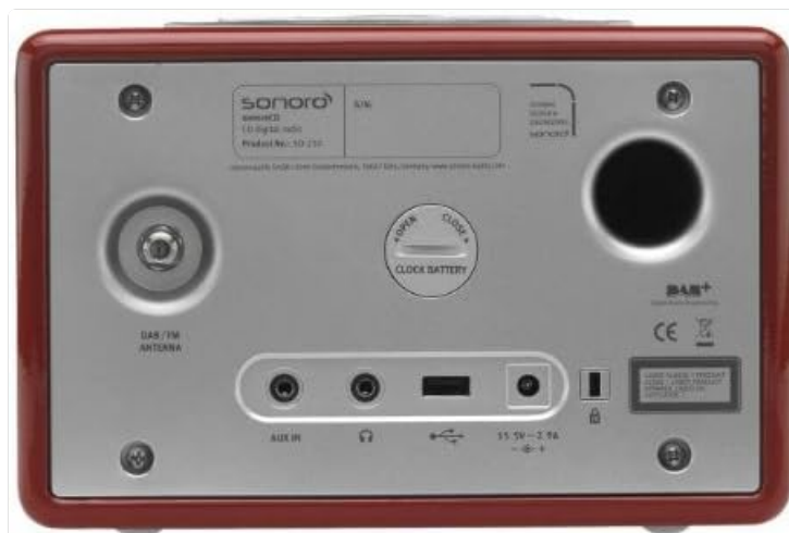
Figure 2: Rear view of the Sonoro SO 2100-100, displaying various connection ports including the antenna input, AUX IN, headphone jack, USB port, and DC power input. The clock battery compartment is also visible.
