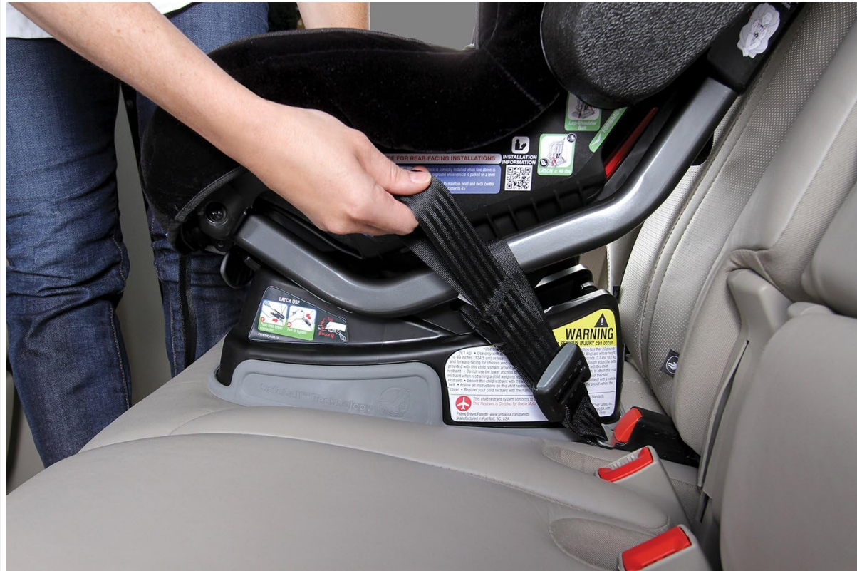
Figure 4.1: Illustrates the process of securing the car seat using the LATCH system. The hand is shown pulling the LATCH strap to tighten the connection to the vehicle's lower anchors.
