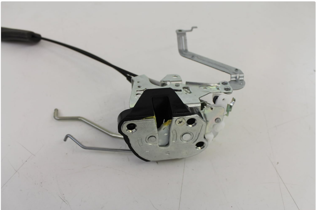
Figure 3: View of the latch side of the sub-assembly, showing the part that engages with the door striker.
