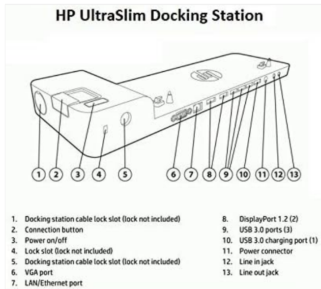
Figure 2.2.6: Comprehensive diagram of the HP UltraSlim Docking Station, labeling all ports and features for easy identification.
