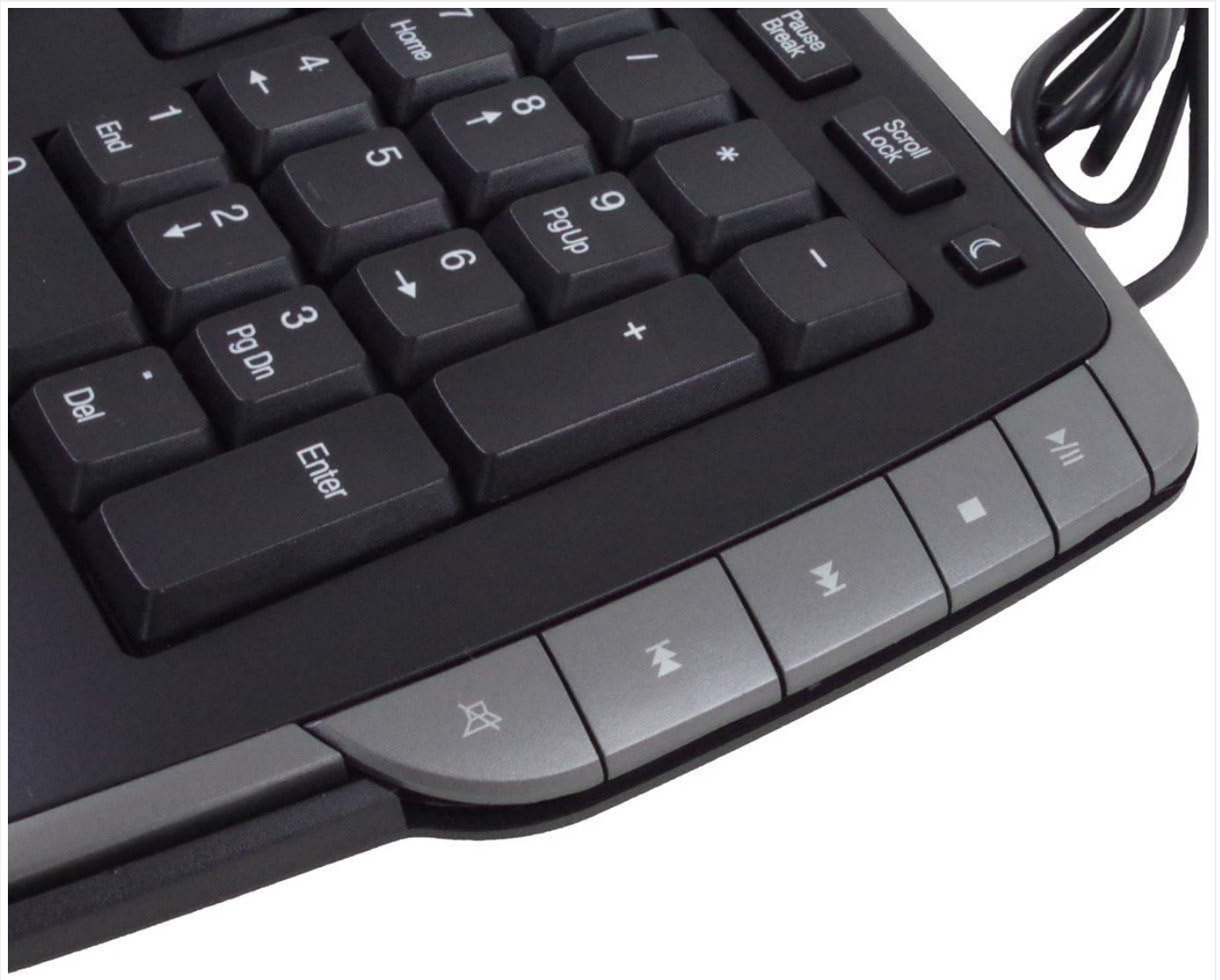
Figure 4.2: Right side view of the keyboard, featuring the numeric keypad and additional multimedia control hotkeys. These keys provide convenient access to media playback controls and other system functions.
