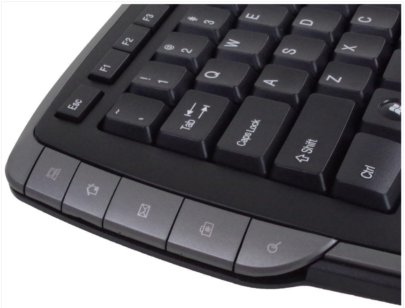
Figure 4.1: Angled view of the keyboard's left side, showing the ergonomic curve and a set of dedicated hotkeys. These hotkeys are typically used for quick access to common computer functions like launching applications or navigating web pages.
