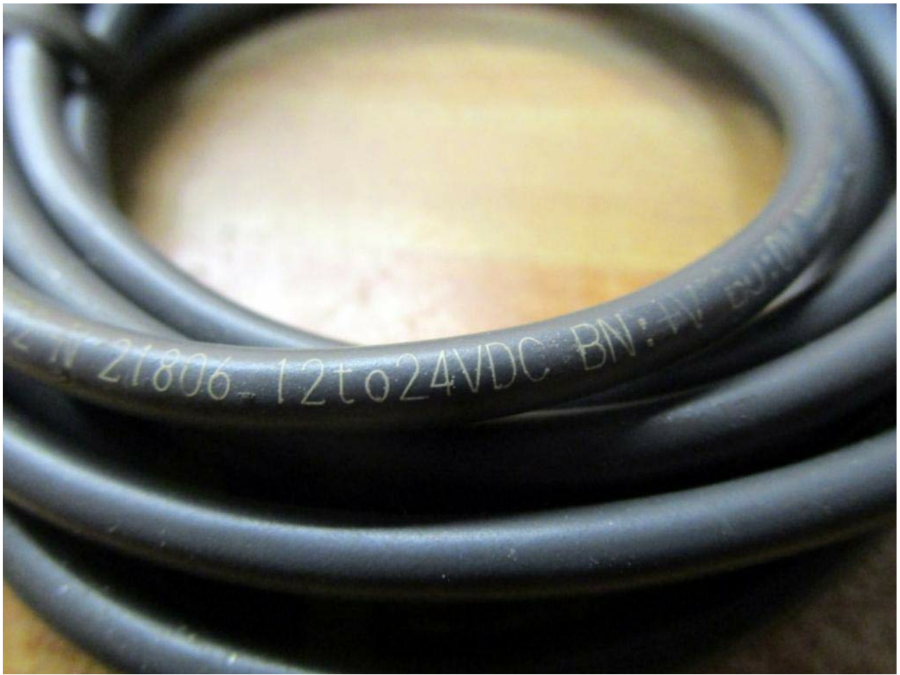
Figure 4.2: Cable marking indicating the operating voltage range "12 to 24VDC".
