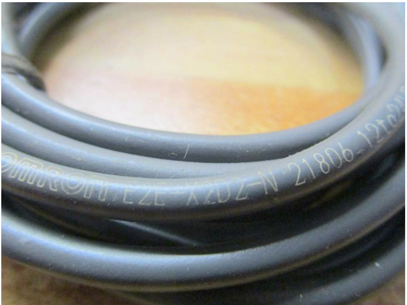
Figure 4.1: Cable marking showing the model number "OMRON E2E X2D2-N".
