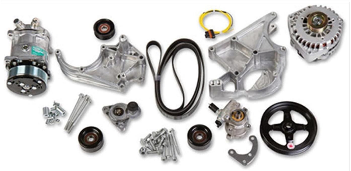
Figure 1: Components of the Holley LS/LT Complete Accessory Drive Kit. This image displays all components included in the Holley 20-137 LS/LT Complete Accessory Drive Kit, laid out on a white background. Key components visible include the air conditioning compressor, alternator, power steering pump, various mounting brackets, pulleys, tensioners, a serpentine belt, and an assortment of bolts and hardware.
