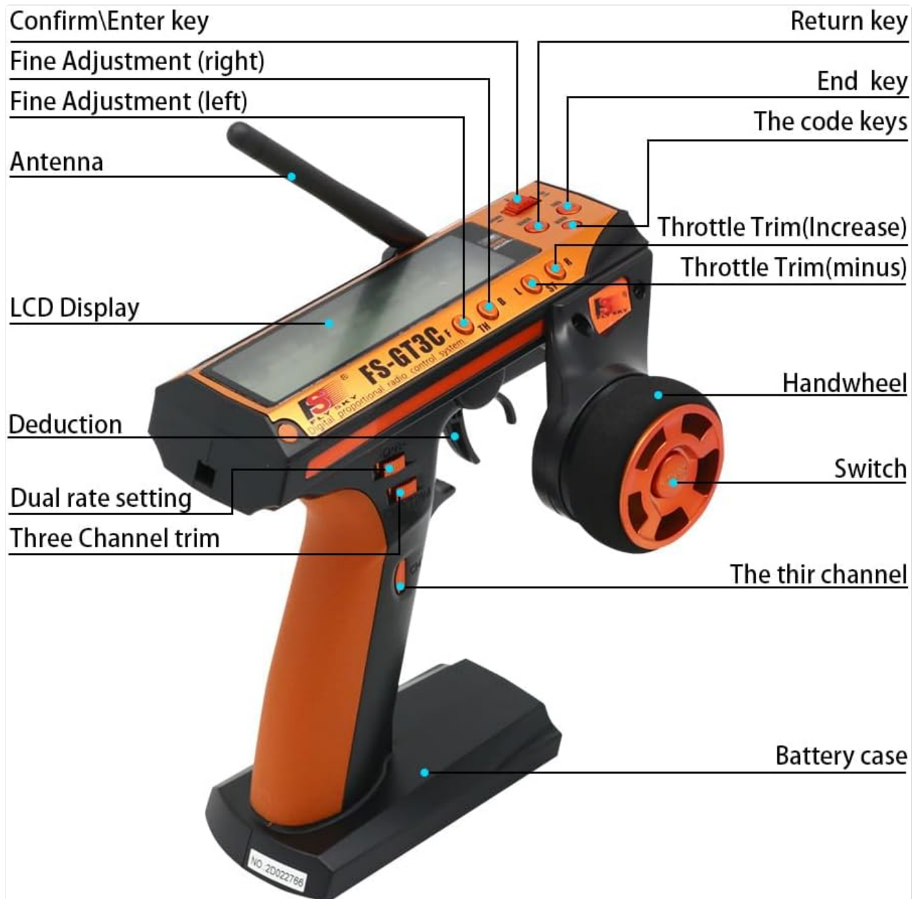
Figure 5.1: Labeled components of the FS-GT3C transmitter.
