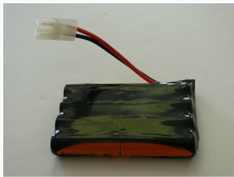
Image: The Banshee Titan 2200mAh 9.6V replacement battery, showing its compact design and connector.
