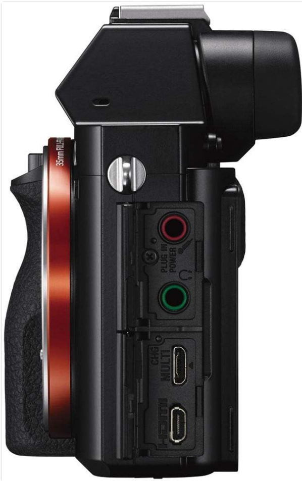
Figure 3.7: Side view of the Sony a7, displaying the various input/output ports including HDMI, USB, and microphone/headphone jacks.
