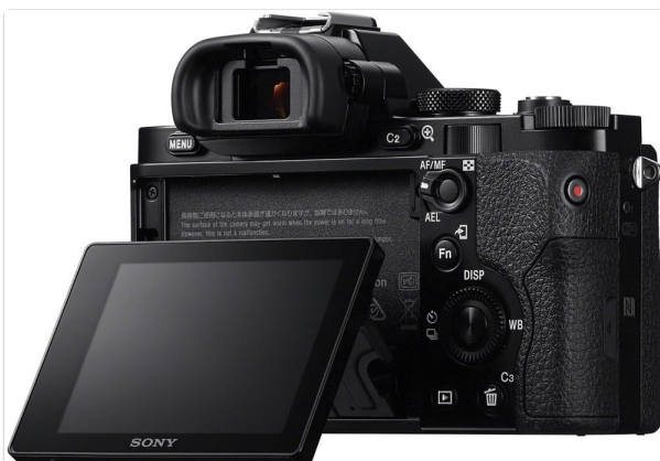
Figure 3.2: Rear view of the Sony a7, displaying the electronic viewfinder, LCD screen, and control buttons.
