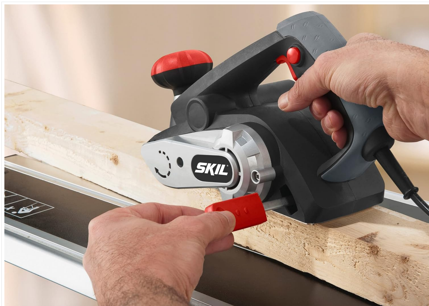
Figure 4.2: Adjusting the planing depth using the front knob. Rotate the knob to select the desired material removal depth.
