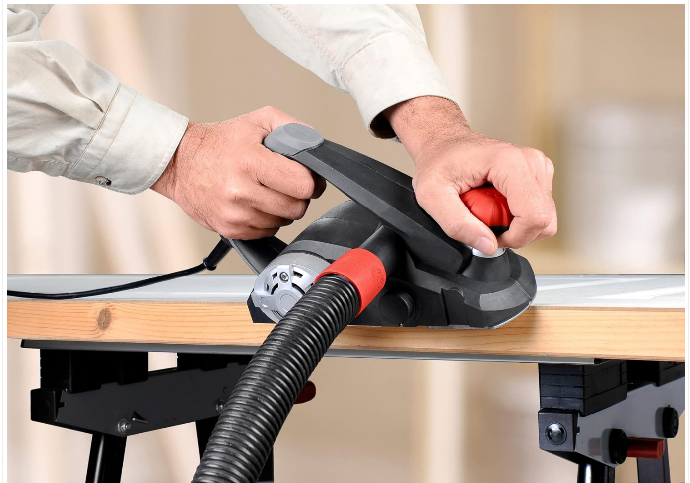
Figure 4.1: Connecting the dust extraction adapter to the planer. This helps manage wood chips and dust during operation.
