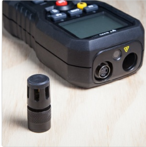
Figure 3.1: The external temperature and relative humidity sensor (MR01).
