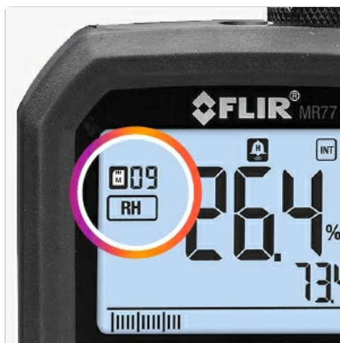
Figure 4.4: The display indicating the selected material group (M09) and Relative Humidity (RH).
