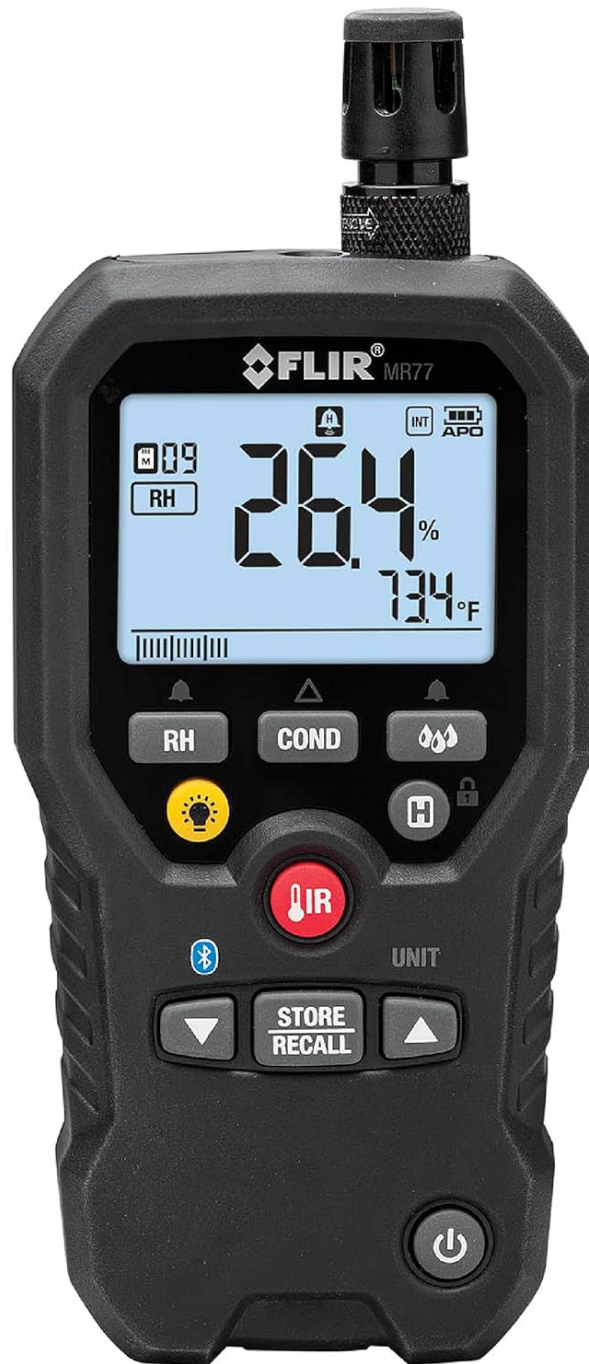
Figure 2.1: The FLIR MR77 Pinless Moisture Meter with its integrated sensor and display.
