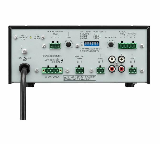
Figure 3.2: Rear Panel of a Representative TOA Power Amplifier (Model BA-260 shown for illustration). This image illustrates the connectivity options, including terminals for MOH (Music On Hold) output, speaker outputs for different zones, line outputs, and various microphone/line inputs. It also shows the power input and a unit breaker reset button.
