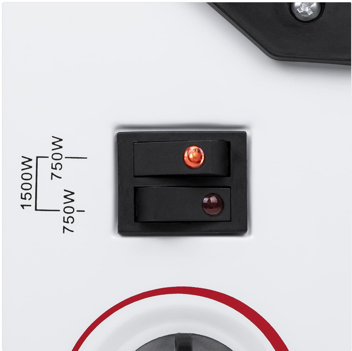
Figure 2: Detail of the power switches. The top switch activates 750W, and the bottom switch adds another 750W for a total of 1500W. Each switch illuminates when active.
