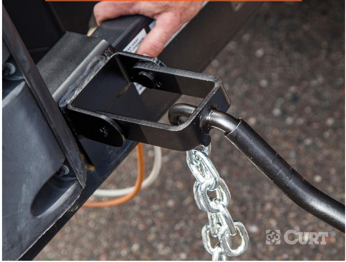
Figure 6: Snap-up brackets facilitate connecting the spring bar chains.
