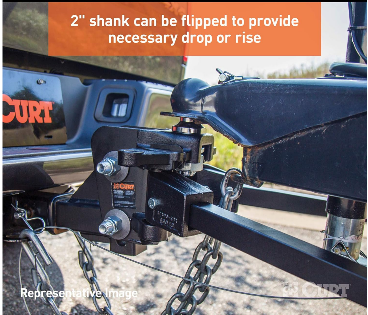
Figure 3: The 2-inch shank can be adjusted for proper height.
