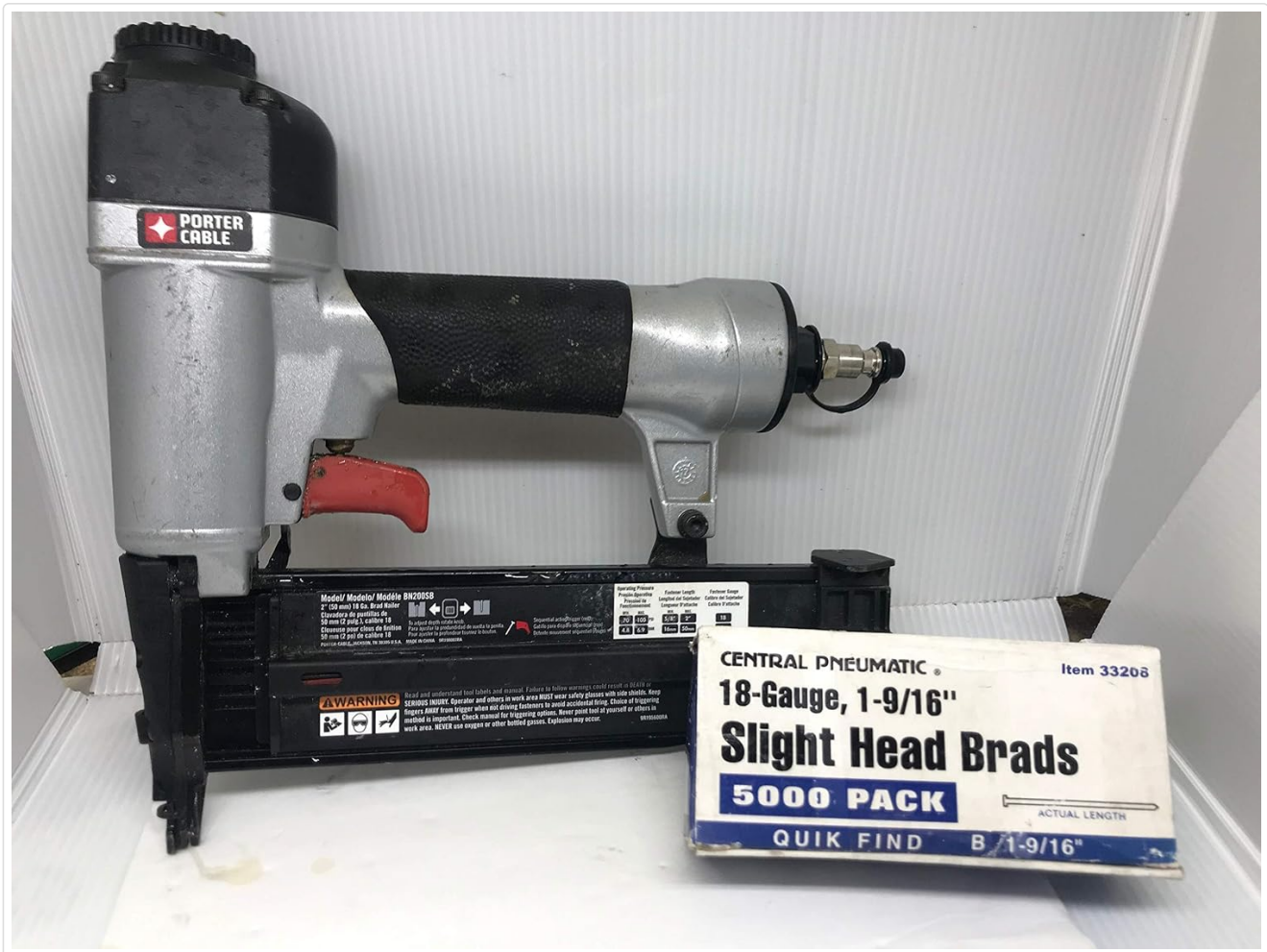
Figure 1: The Porter-Cable BN200SB Brad Nailer. Note the air inlet fitting at the rear of the handle for connecting to an air compressor.
