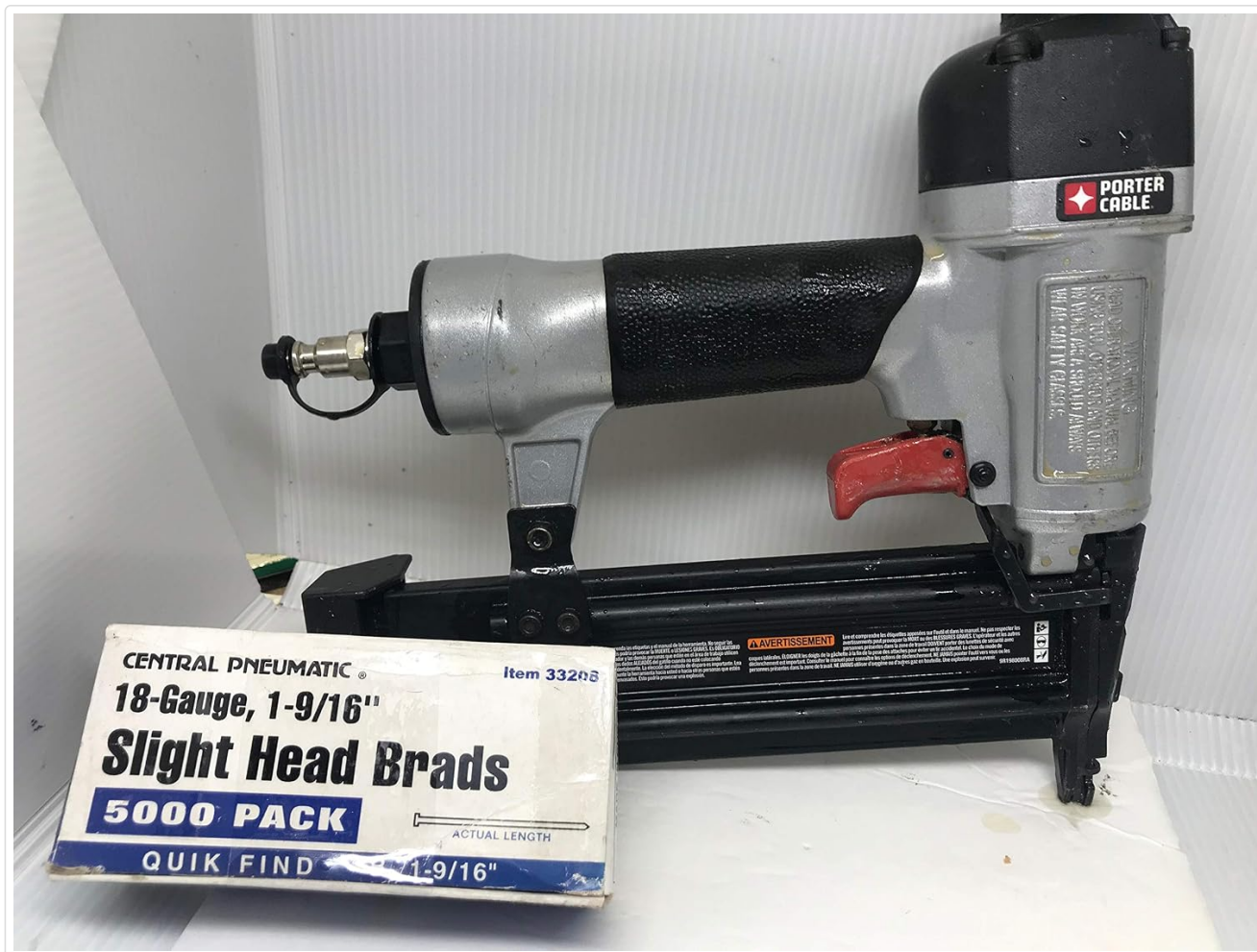
Figure 2: The Porter-Cable BN200SB Brad Nailer shown with a box of 18-gauge brad nails, illustrating the type of fasteners used with this tool.
