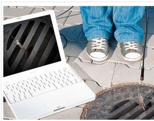
Image: The endoscope camera in use, displaying a live view from inside a manhole on a laptop screen. The cable extends into the manhole, demonstrating its application for inspecting confined spaces.
