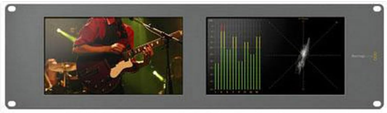
Figure 2: Front panel displays. This image shows the two independent screens, with one displaying a video feed and the other showing a vectorscope or similar analysis tool.
