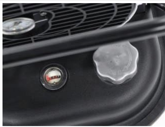
Image 3: Detail of the fuel cap and integrated fuel level indicator for easy monitoring.
