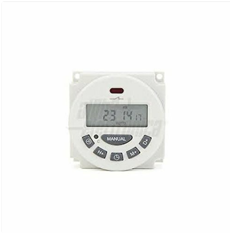
Figure 1: Front view of the Lafayette TDS-12 Digital Timer. This image shows the digital display and control buttons.
