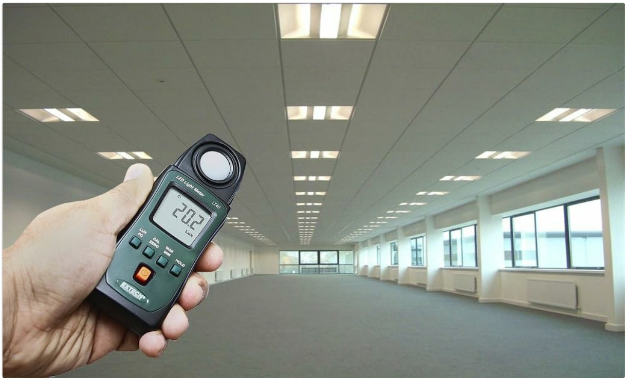
Figure 2: Measuring light levels with the Extech LT40
