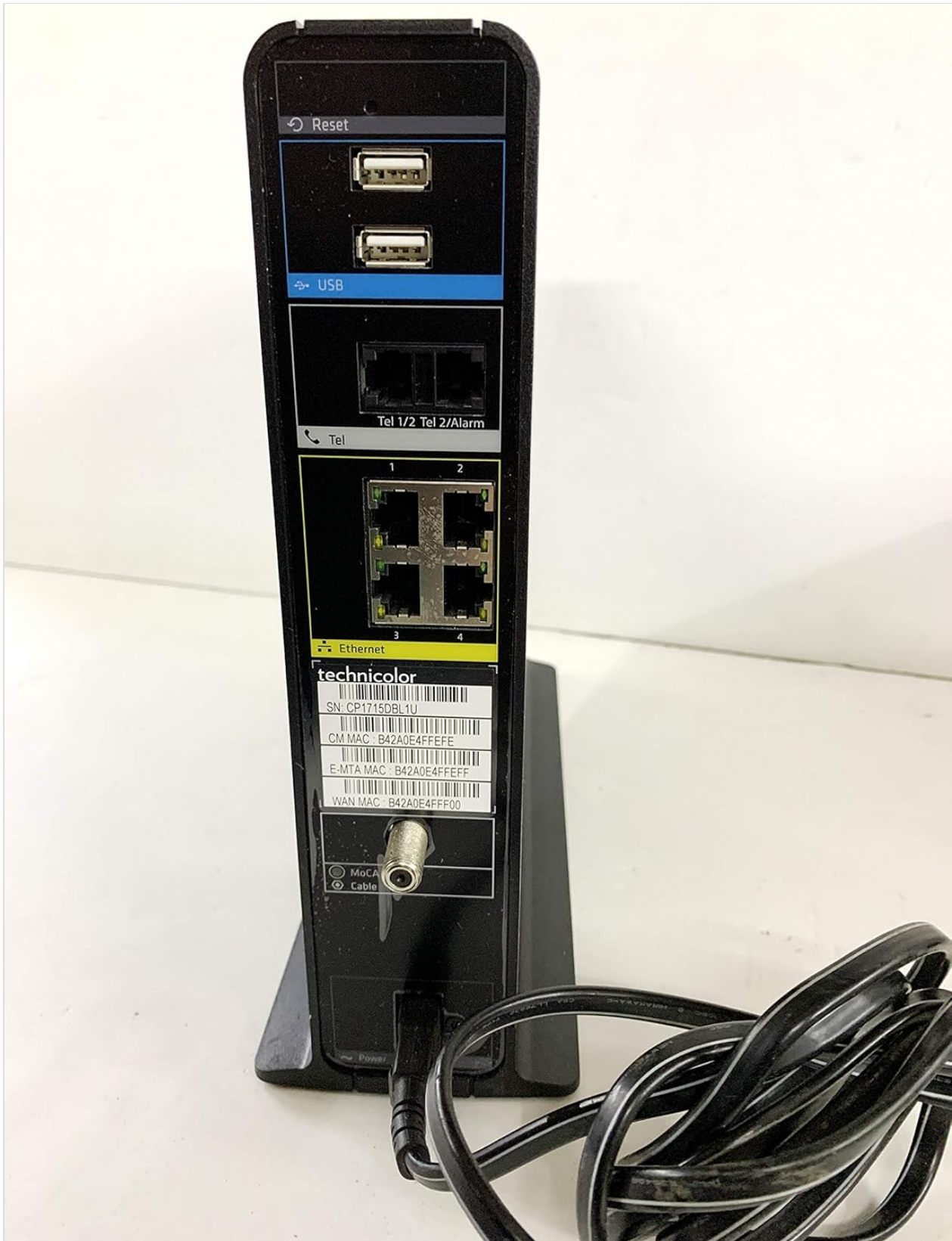
Rear view of the Technicolor TC8717T modem router, highlighting the coaxial, Ethernet, USB, and telephony ports, along with the power input and On/Off switch. This view is essential for connecting all necessary cables during setup.
