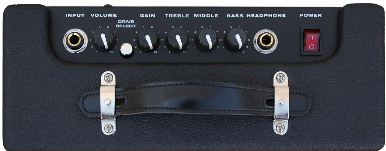
Figure 4: Amplifier Control Panel.
