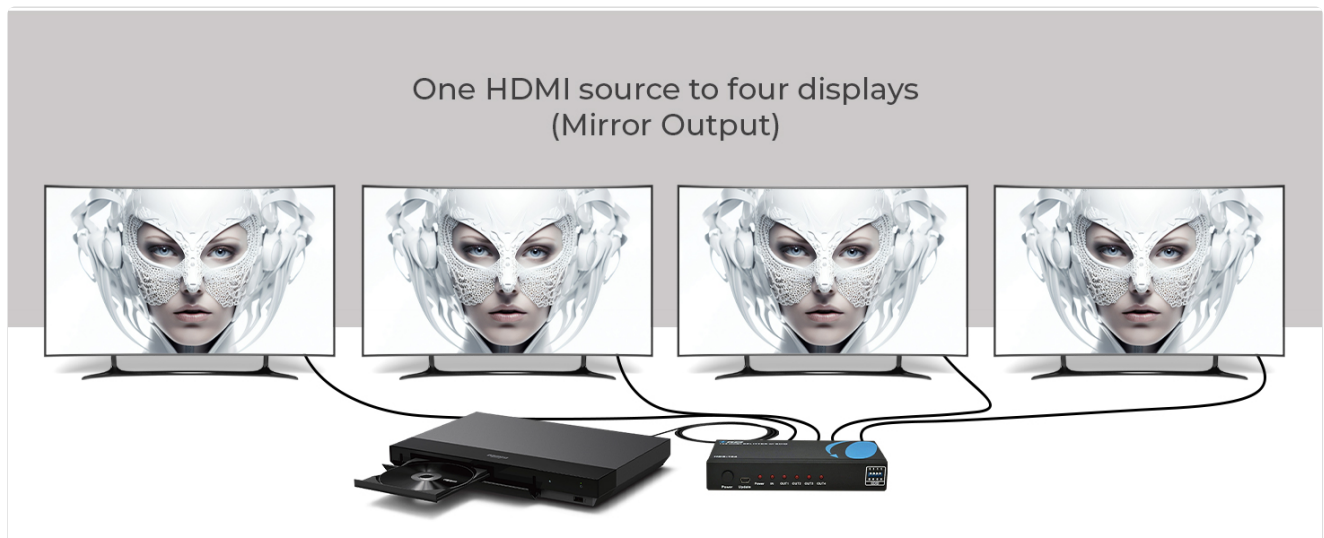
Figure 4: Typical connection diagram for the OREI HDS-104.
