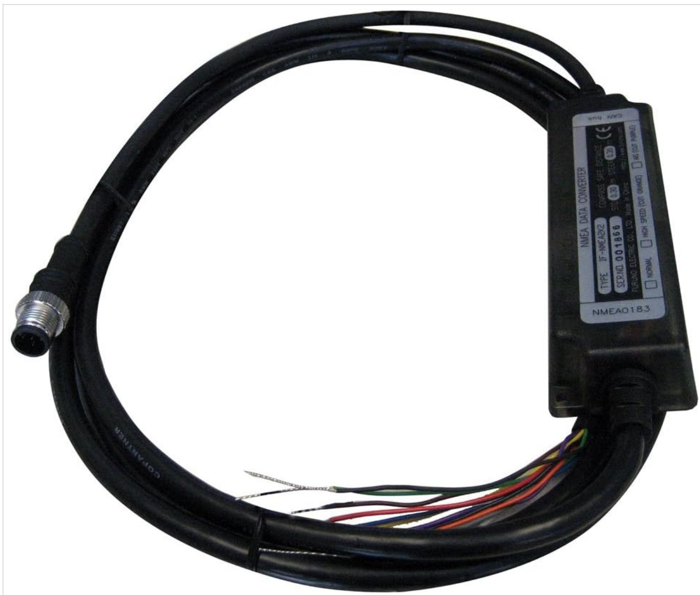
Figure 1: FURUNO FUR-IF-NMEA2K2 NMEA Data Converter. The image displays the converter unit with a circular NMEA 2000 connector on one end and multiple color-coded bare wires for NMEA 0183 connections on the other. The main body of the converter is black with a label indicating "NMEA DATA CONVERTER", "TYPE IF-NMEA2K2", "SER.NO. 001866", and options for "NORMAL" or "HIGH SPEED (CUT ORANGE)" operation.
