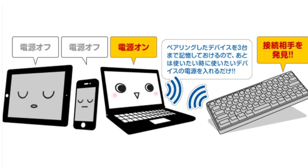
Image: A diagram showing the keyboard's ability to connect to and switch between three Bluetooth devices.
