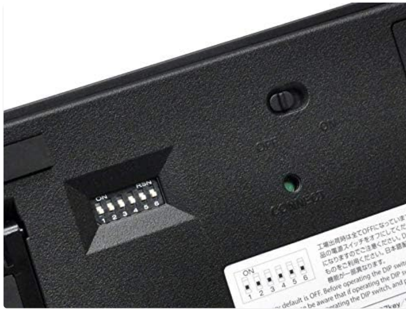
Image: The underside of the keyboard showing the battery compartment and DIP switches.
