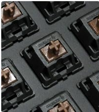
Image: A close-up view of the Cherry MX Red mechanical switch, known for its linear feel.
