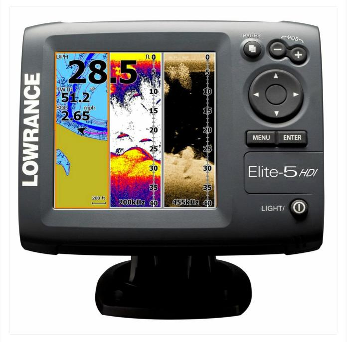
This image displays the Lowrance Elite-5 HDI Combo unit. The screen shows a split view: a chartplotter on the left with navigation data, and two sonar views on the right, indicating depth and underwater structures at 200kHz and 455kHz frequencies. The unit features a keypad with directional buttons, MENU, ENTER, PAGES, MOB, and LIGHT/POWER buttons.
