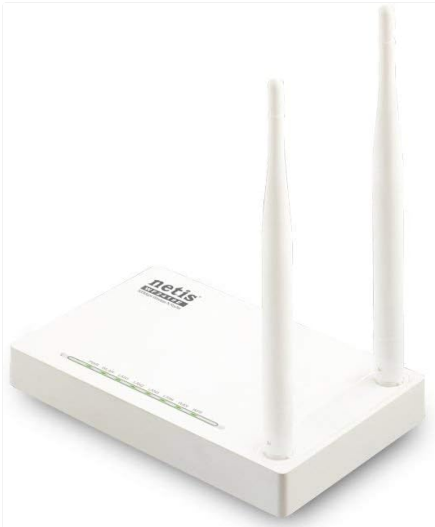
Figure 2.3: Front view of the Netis WF2419 router, showing the LED indicators that provide status information for power, wireless activity, WAN connection, and LAN port activity.
