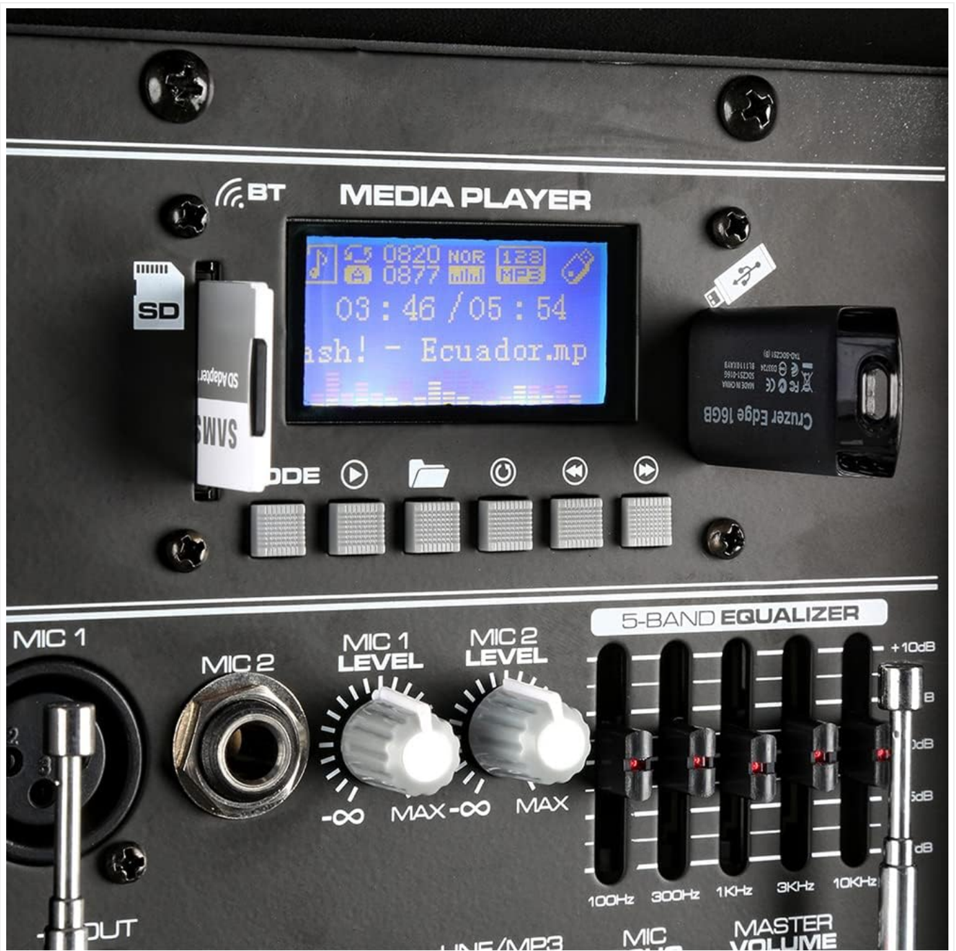
Figure 2: Detailed view of the control panel, showing the media player display, USB/SD card slots, microphone level controls, and the 5-band graphic equalizer.
