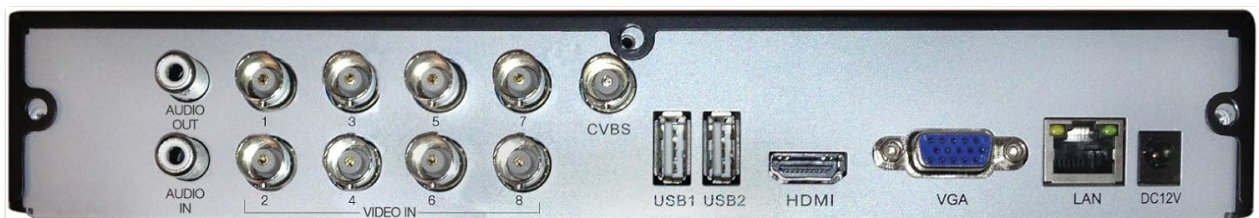
Figure 2: Rear panel of the Q-See QT228-8B5-5 DVR. This view shows the audio input/output ports, eight BNC video input ports, CVBS output, two USB ports, HDMI output, VGA output, LAN port, and DC12V power input.
