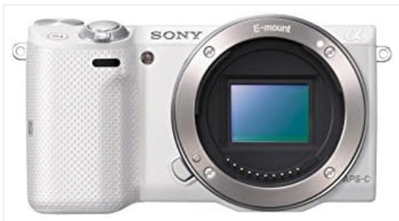
Front view of the SONY NEX-5T camera body without the lens, revealing the E-mount for interchangeable lenses and the APS-C sensor.
